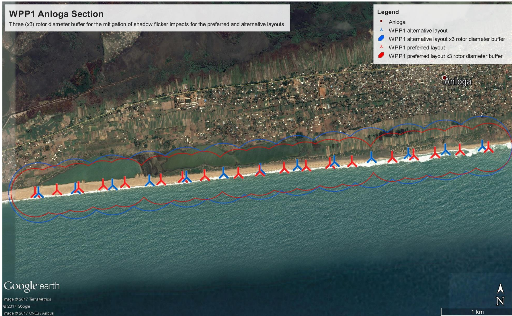
Figure 7-16: Three rotor diameter buffer for the Anloga section of WPP1, for shadow flicker impact mitigation
