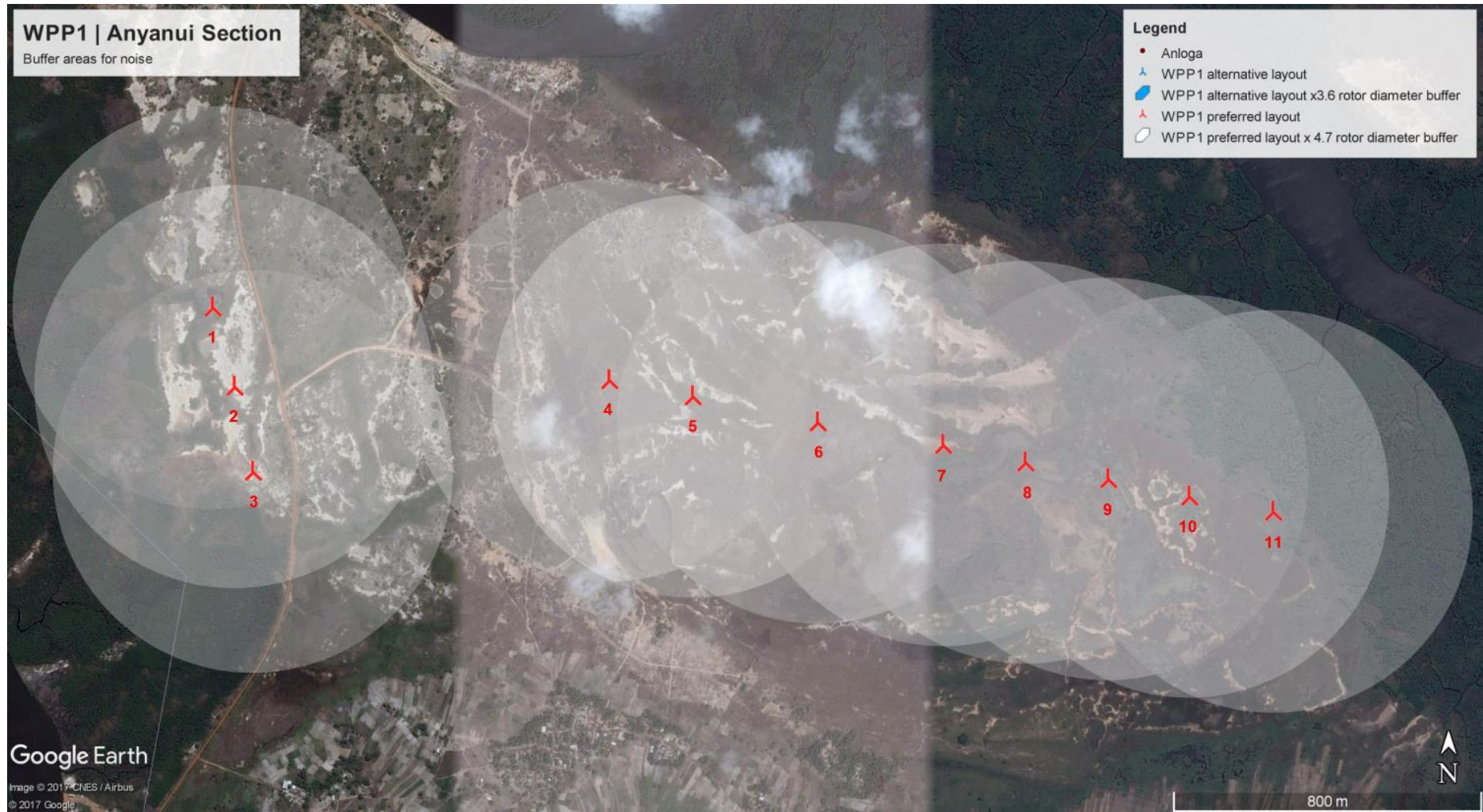
Figure 7-12: Buffer for the Anyanui section of WPP1, for noise impact mitigation
