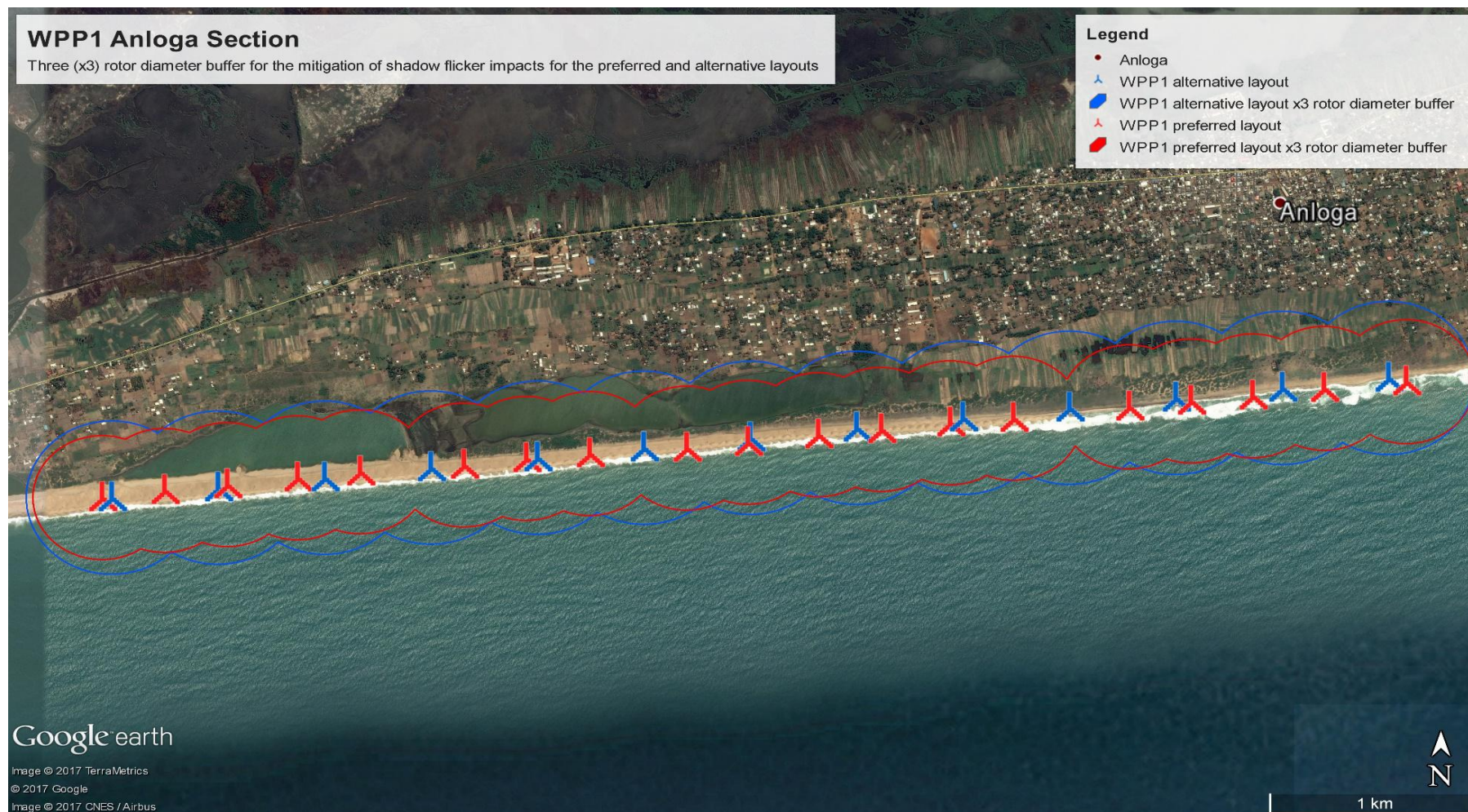
Figure 4: Three rotor diameter buffer for the Anloga section of WPP1, for shadow flicker impact mitigation
